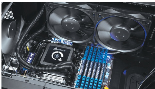
COOLING is provided by a Digital Storm Vortex liquid cooling system.
